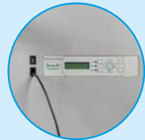
Control panel separated from robot for redundancy safety
